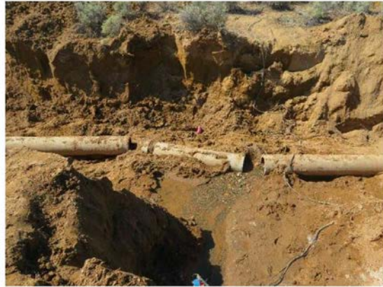
Damage to buried pips in 2019 M7.1 Ridgecrest event
